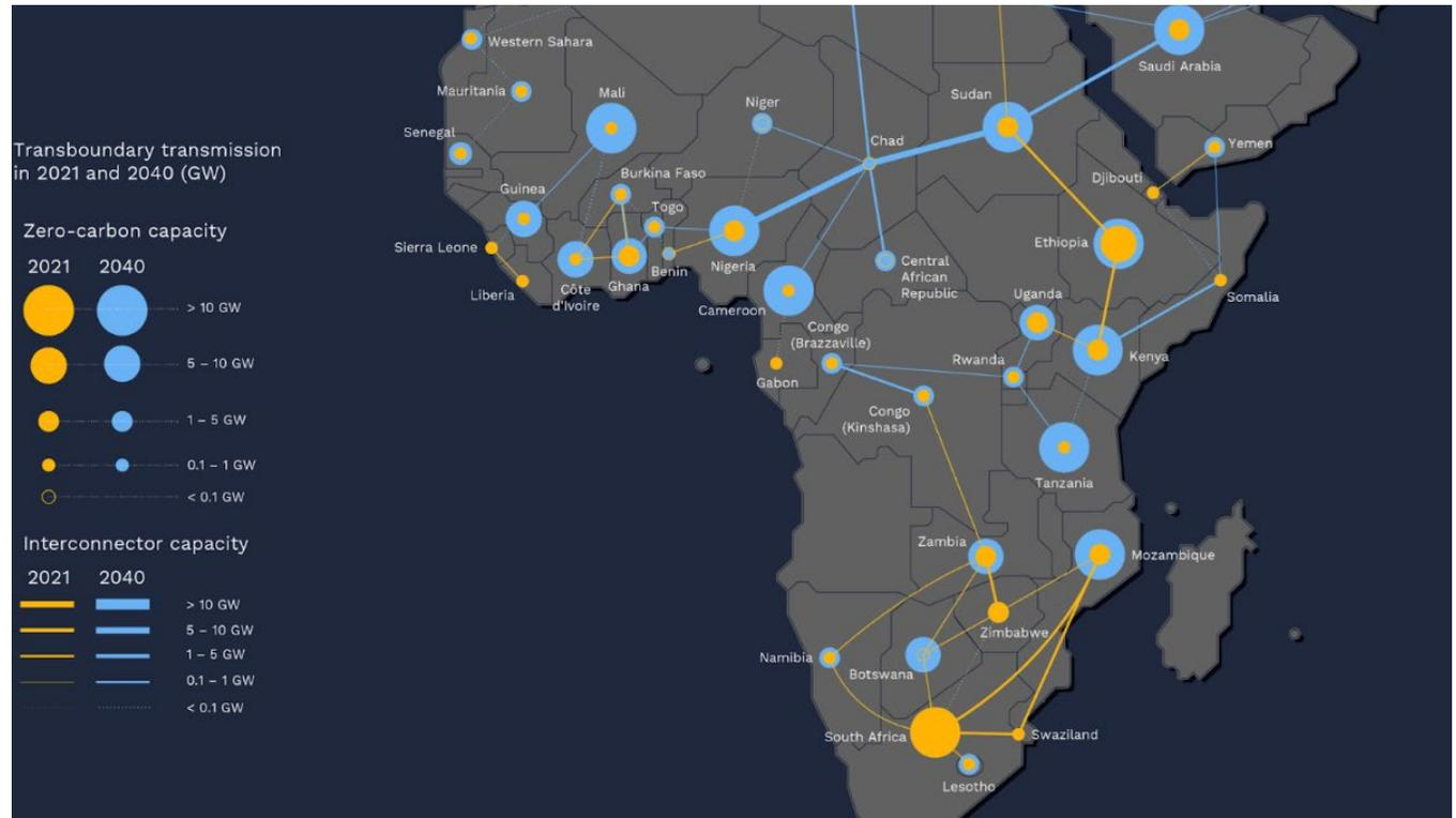
Figure 5 - High-level example of grid simulation at regional level, visualising the contribution of interconnections to the increase of zero carbon capacity (Source: TransitionZero, 2023)
